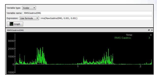
3. The maximum value of the RMS signal can then be calculated using the max(X, StartTime, StopTime, Interval) operator, which defines the maximum value for a Scalar, X, that occurred over a time period defined by StartTime and StopTime, and Interval that is the step size (in seconds) for evaluating your time period.
