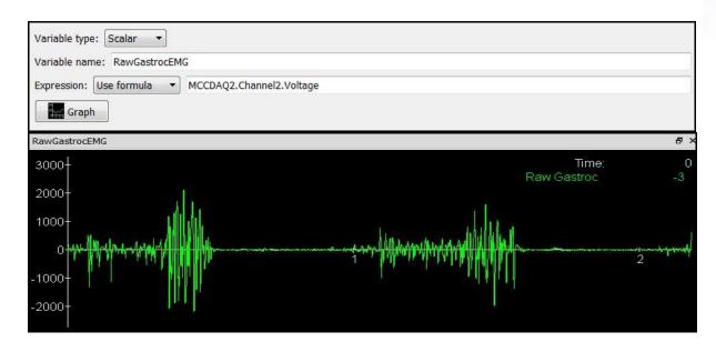
When collecting analog signals, the **AnalogEMG** device under the hardware node can be enabled. This allows the user to output the root mean squared (RMS) signal directly. If this has been configured step 2 can be skipped.
