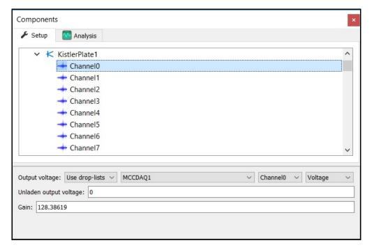
4. From the Kistler plate parameters panel click the "Calibrate" button to perform a software zero and click on the "Align" button to begin the procedure for aligning the force plate to the world axes.
