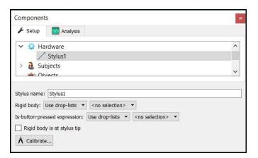
Once all parameter fields are completed, click the "Calibrate" button and follow the prompts to calibrate your stylus. A tutorial video for configuring the stylus can be found at <a href="https://themotionmonitor.com/support/">https://themotionmonitor.com/support/</a>.
