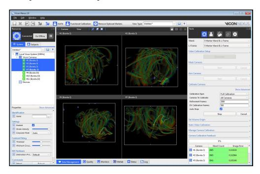
5. Now place the wand at the origin of the global coordinate system. Ensure that all 5 markers can be seen by each camera. Expand the "Set Volume Origin" dropdown. Click "Start" and then "Set Origin" when you are ready to take a reading. **Note:** It's important to place and orient the wand in an identical manner from calibration to calibration, to ensure that any force plate alignments remain valid relative to Vicon's origin.
