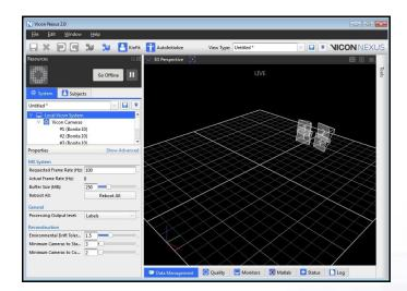
2. Next, highlight all the cameras within the System tab in the Resources pane, and select "Camera" view from the "Camera" dropdown in the Animation pane. At this time, all efforts should be made to eliminate unwanted reflections. If required, camera pixels can be masked automatically using the "Create Camera Masks" function in the Tools pane under System
