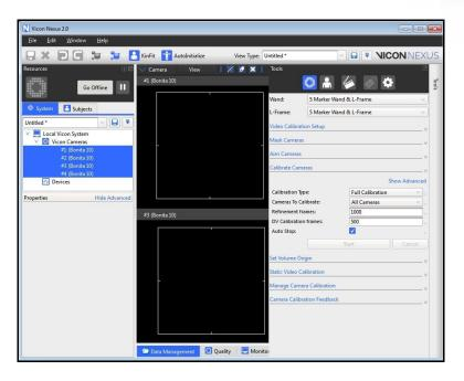
4. Move the wand throughout the measurement volume, being sure to move in all three axes. The camera view will display the area that has been covered with a rainbow, and the Wand Count will update as frames are collected. Once all of the cameras have recorded at least the required number of Refinement Frames, the calibration will be calculated. Note: It's important that the Refinement Frames for each camera update at a uniform rate, in order to ensure good calibration coverage.
