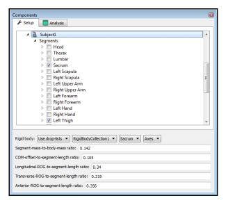
19. Each body segment which is enabled will require the definition of a proximal and distal endpoint or joint centers. The required joint centers will be automatically populated based on the selection of segments.
