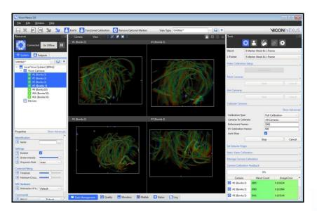
5. Now place the wand at the origin of the global coordinate system. Ensure that all 5 markers can be seen by each camera. Expand the "Set Volume Origin" dropdown. Click "Start" and then "Set Origin" when you are ready to take a reading.
