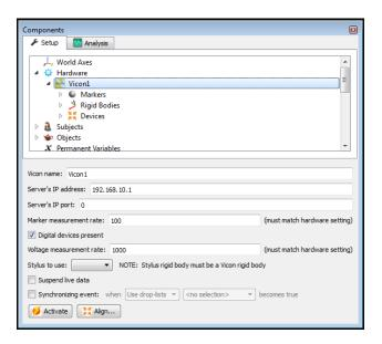
14. After successfully activating the Vicon device, the marker list, rigid bodies list and any analog data configured within Vicon will be populated under the appropriate headers for the Vicon component. Data repair and smoothing settings can be enabled or disabled here, pre or post data collection.
