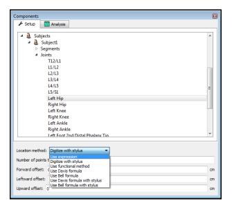
20. As seen above, each joint center can be defined using a digitizing method or expression based on marker positions. Alternatively, the hip and shoulder joints can be defined using linear regression algorithms or functional (rotational) methods.
