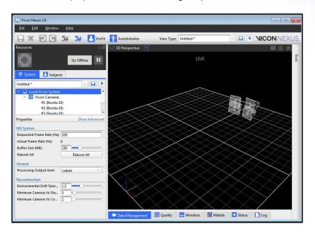
2. Next, highlight all the cameras within the System tab in the Resources pane, and select "Camera" view from the "Camera" dropdown in the Animation pane. At this time, all efforts should be made to eliminate unwanted reflections. If required, camera pixels can be masked automatically using the "Create Camera Masks" function in the Tools pane under System Preparation () or manually using the masking icons in the Animation pane.
