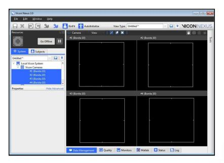
3. Now, begin the calibration process. From Tools, go to System Preparation ( ). Ensure the appropriate Wand and L-Frame are selected (i.e. "5 Marker Wand & L-Frame") and then
