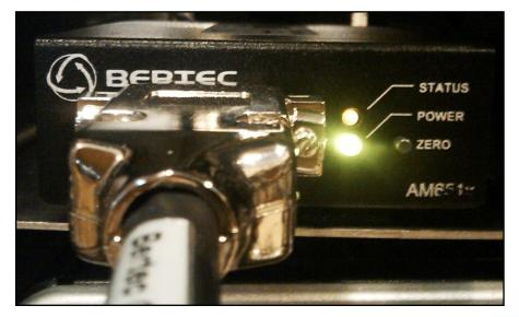
5. Connect the power supply to the Amplifier.
