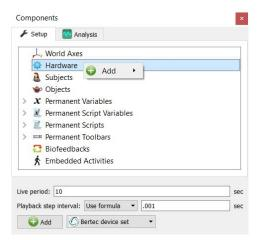
4. Click on the Bertec device set to bring up the parameters panel. Set the measurement rate to 1,000 (Hz). The suspend live data checkbox will suppress any data from the Bertec device from being displayed in graphs or used in any equations. However, the data would immediately be available and presented in a recorded activity. This is a means for limiting the computer resources being used while running in the Live Window.
