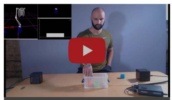
Polhemus VIPER™ sensors are attached to the subject's trunk, upper arm, hand, index and thumb fingers. A biomechanical model of the upper extremity, including hand & fingers, is defined within The MotionMonitor xGen software. Skeletal animation and data graphs are displayed in real-time, allowing the researcher to quality check data as it is collected. Advanced user-defined analysis, including bar & time series graphs, musculoskeletal animation and text, can then be loaded quickly with an icon.
